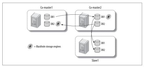
Figure 8-13. Emulating multimaster replication with dual masters and the Blackhole storage engine
