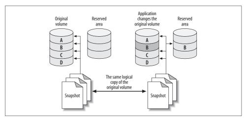
Figure 11-1. How copy-on-write technology reduces the size needed for a volume snapshot
