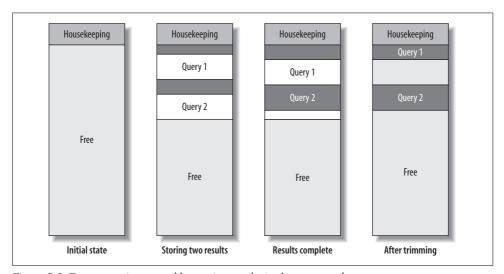
Figure 5-2. Fragmentation caused by storing results in the query cache
