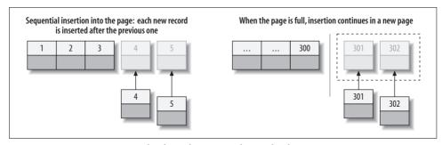
Figure 3-10. Inserting sequential index values into a clustered index
