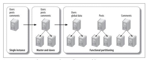
Figure 9-2. From a single instance to a functionally partitioned data store
