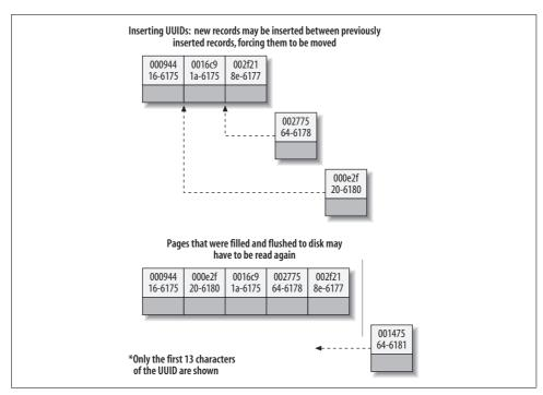
Figure 3-11. Inserting nonsequential values into a clustered index
