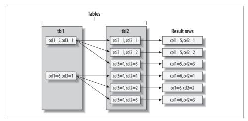
Figure 4-2. Swim-lane diagram illustrating retrieving rows using a join
